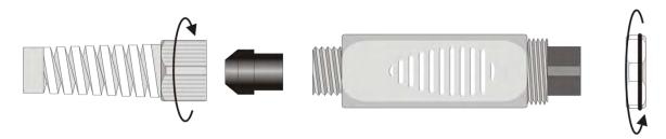
Open the two module shells: the printed circuit to which the probe must be connected is housed inside. On the left there are the 1...4 points on which the sensor wires must be welded. The JP1...JP4 jumpers are in the center of the board. These must be closed with a tin bead for some type of sensors:
