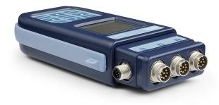
The instrument is provided with three inputs for probes with SICRAM module: the SICRAM module is an interface between the instrument and connected sensor and communicates the sensor parameters and calibration data to the instrument. All SICRAM probes can be plugged into any of the inputs: they are automatically recognized upon turning on the instrument.
