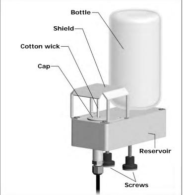
For measurements in presence of solar irradiation, use the protection shield from solar radiations. Note: over time the cotton wick tends to calcify (harden): it must be replaced periodically.
